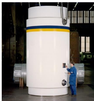
Figure 6 : A Dry Storage Cask for Medium Term Fuel Assembly Storage
