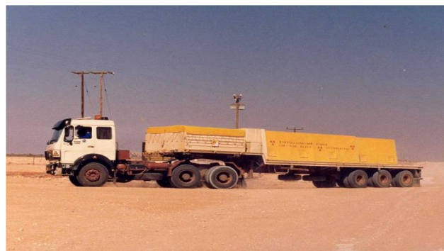
Figure 3 : LLW and ILW Pack into Sealed Containers on Transport to Vaalputs
