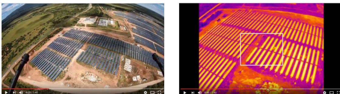
**Figure 8:** Typical infra-red image of a photovoltaic plant with the PV panels at an elevated temperature (yellow areas): (a) Daylight image; (b) Infra-red image.
