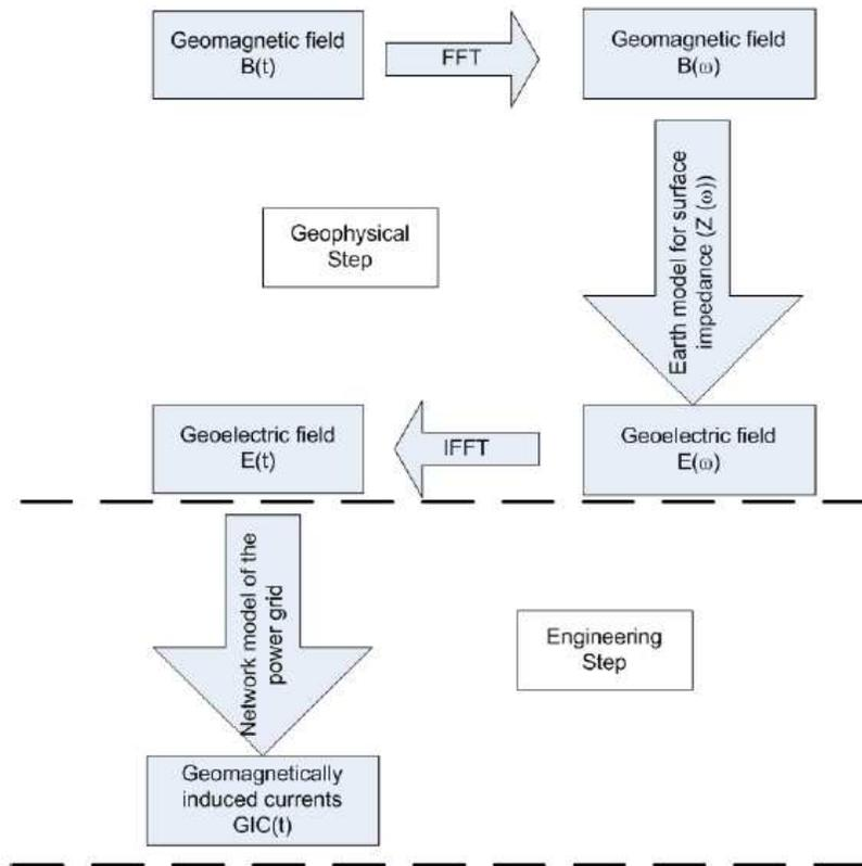
Figure 1. Frequency domain approach for finding the geo-electric field for the estimation of GICs in power lines from geomagnetic and surface impedance data. Adapted from (Zheng et al., 2013 [13]).
