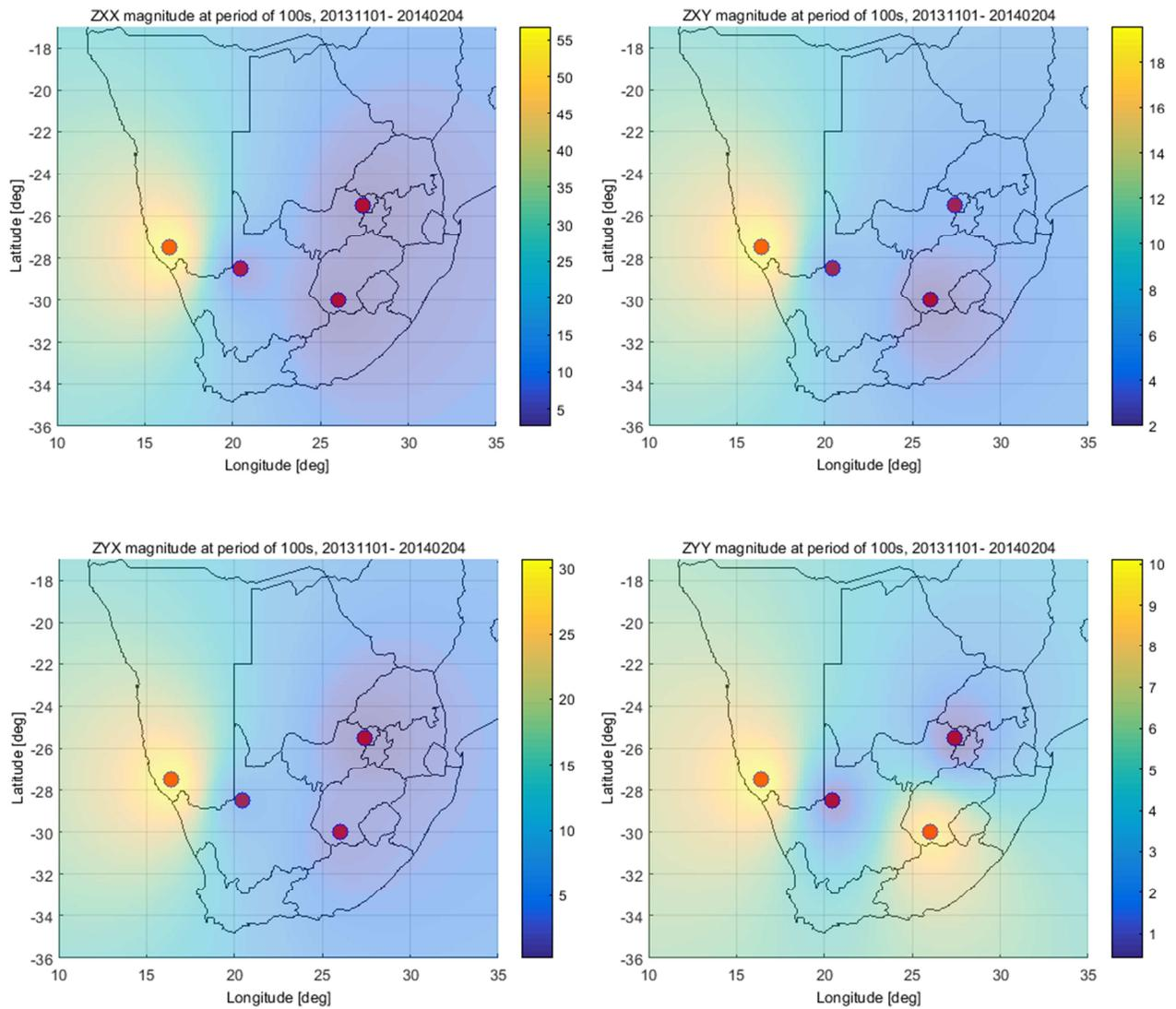
**Figure 4. Examples of the interpolation of the surface impedance over Southern Africa based on the simultaneously measured surface impedance values at four MT stations Hartbeesthoek (27.42°E, 25.53°S), Obib (16.38°E, 27.51°S), Kakamas (20.46°E, 28.49°S) and Trompsburg(26.01°E, 30.07°S).**
