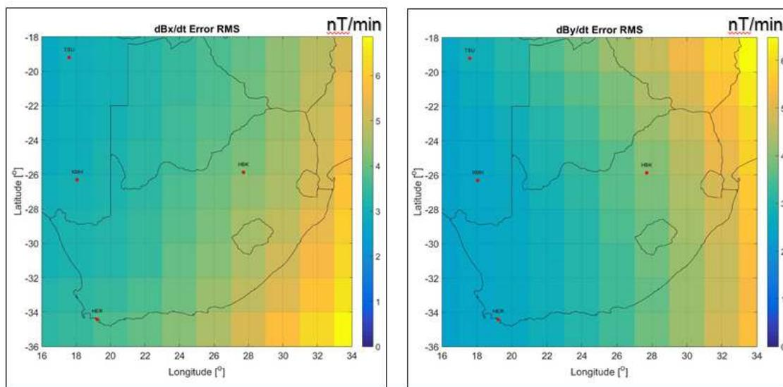
**Figure 3. Plots of the RMS error, in nT/min, for  $dBx/dt$  (Left) and  $dBy/dt$  (Right), between SWMF simulated and interpolated values, averaged over the duration of the simulated fields for the geomagnetic storm on 2003-11-20, at each point on a 2 x 2 degree grid. The locations of the INTERMAGNET magnetometer stations are shown on the maps. The simulated data from these stations were used for the interpolation using the SECS method.**
