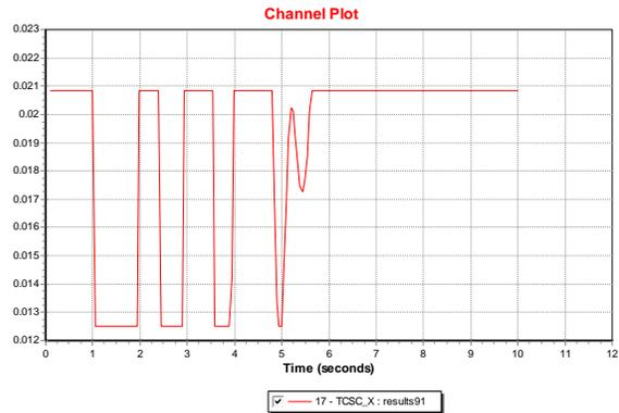
Figure 12: Medupi-Marang line reactance (TCSC output)
