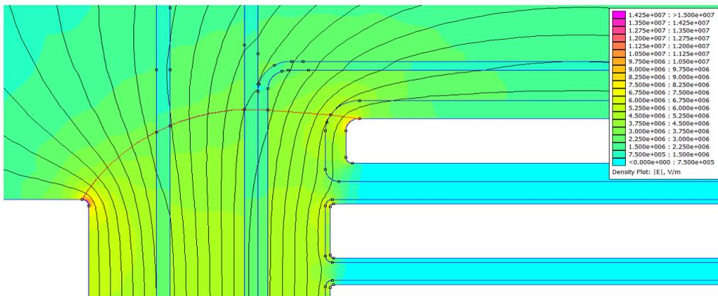
**Figure 54 Electric Field Intensity in Mineral Oil Transformer**
