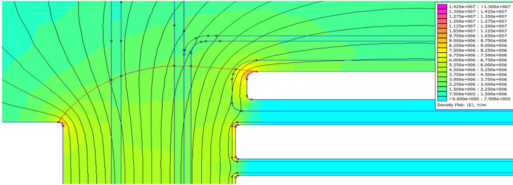
Figure 65 Electric Field Intensity in Natural Ester Oil Transformer
