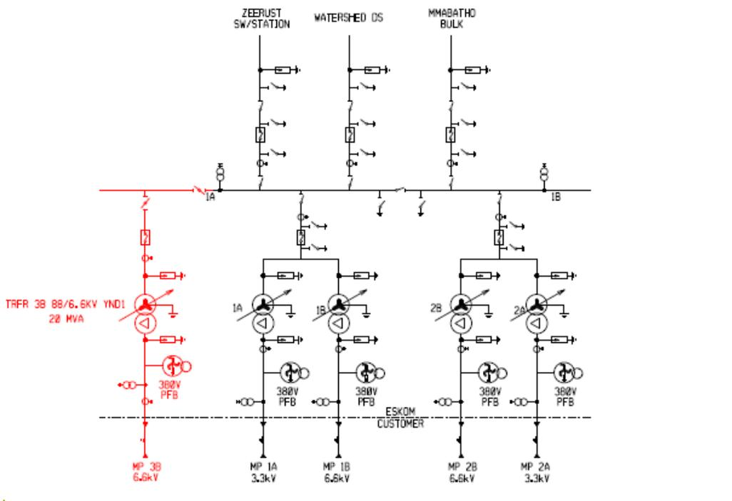
Figure 1 Station Diagram of PPC Slurry Substation
