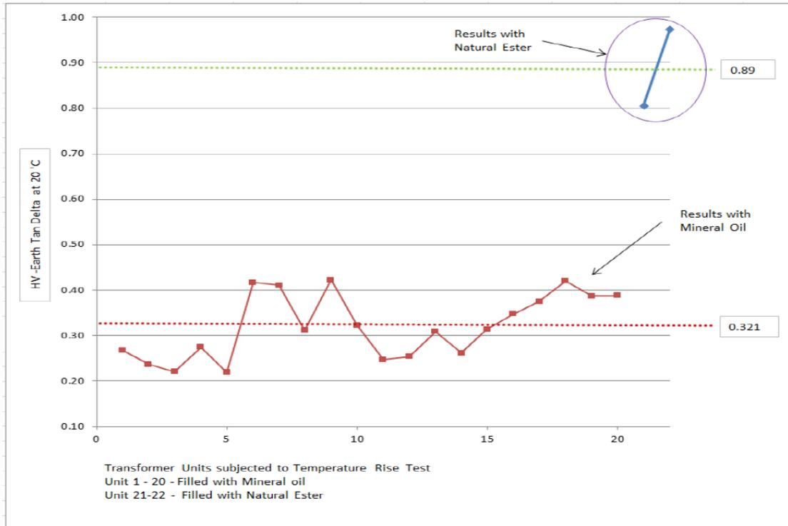
**Figure 2: Comparison of winding tan delta values between identical designs of mineral oil and ester liquid filled transformers**
