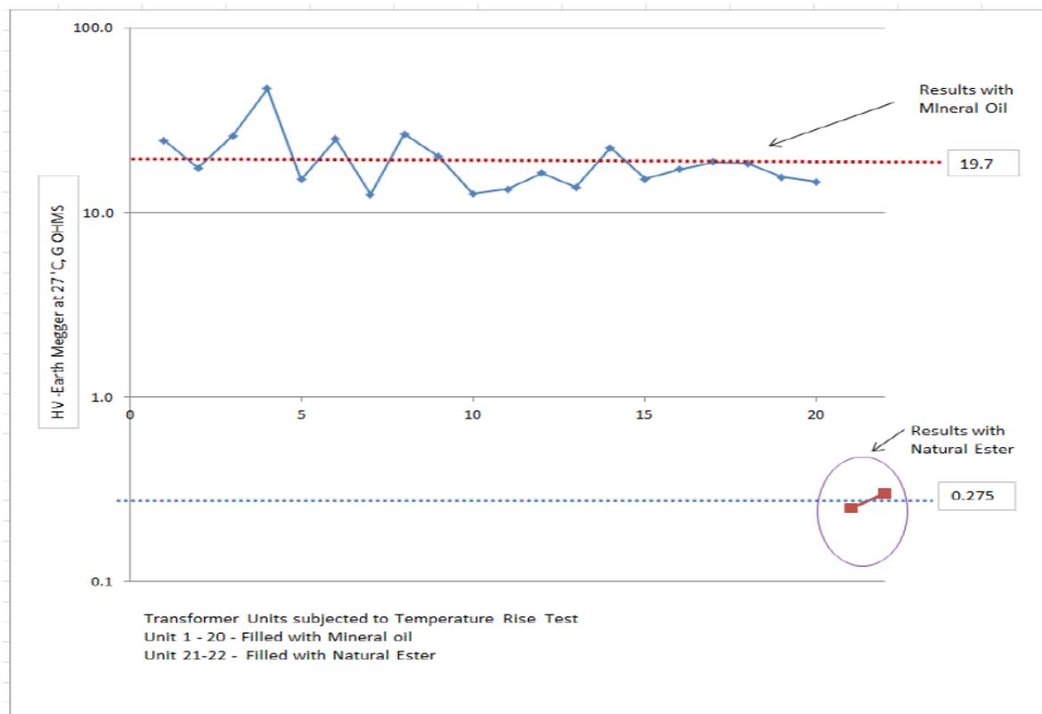
**Figure 1: Comparison of insulation resistance values between identical designs of mineral oil and ester liquid filled transformers**
