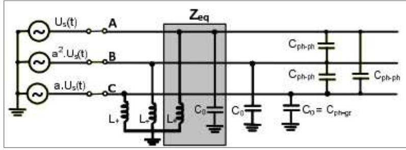
Figure 1: Application of shunt line reactor [2]
