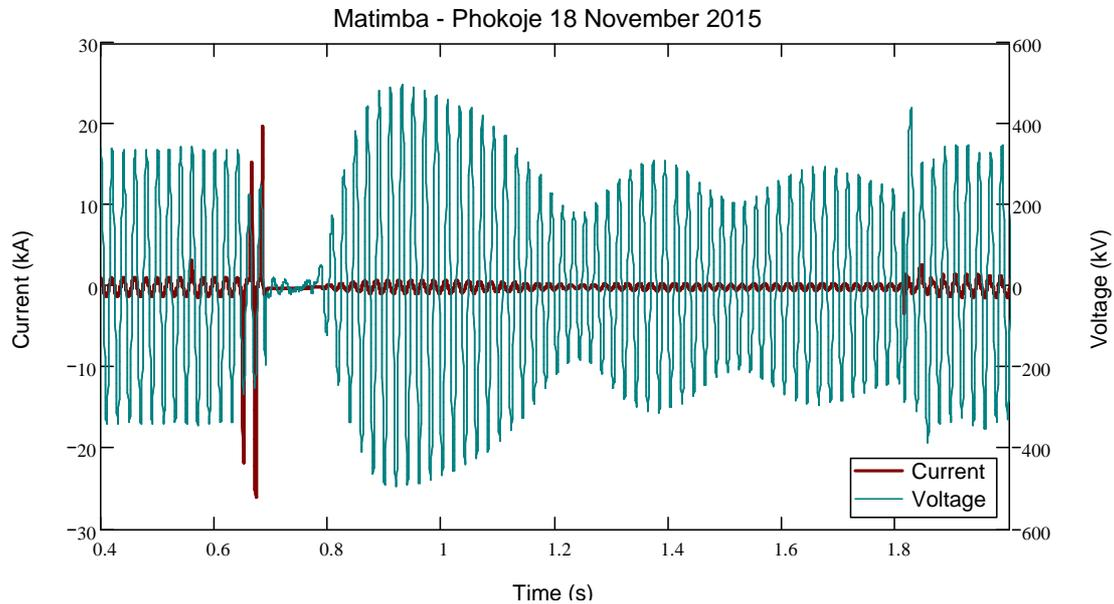
Figure 7: Matimba - Phokoje fault recording (Without NER) 18 November 2015
