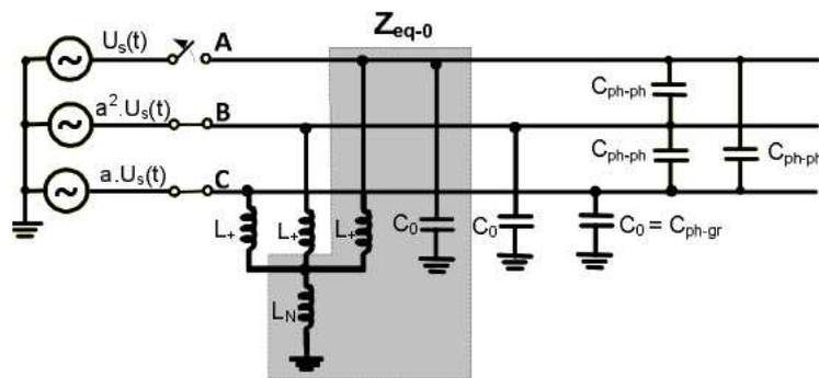
Figure 2: Neutral Earthing Reactor
