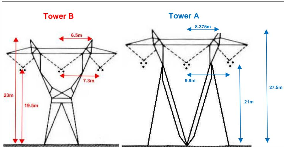
Figure 3: 400 kV Transmission line geometries
