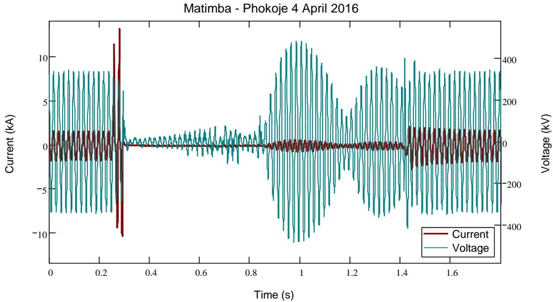
Figure 6: Matimba - Phokoje fault recording (Without NER) 4 April 2016
