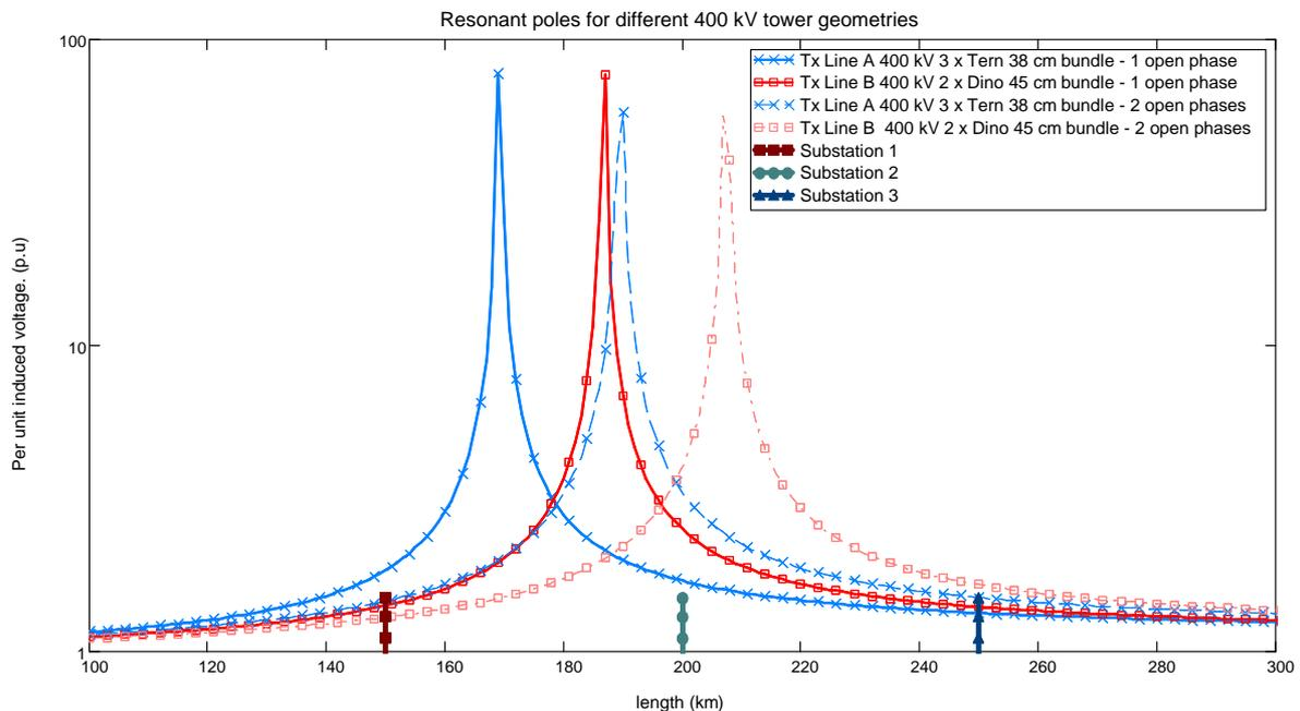
Figure 4: Resonant Pole plot for Line A and B as a function of line length
