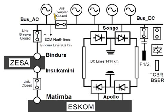
Fig. 2: Simplified diagram of the interconnection between HCB and Eskom. Source: Goosen et. al. (2003) [10]
