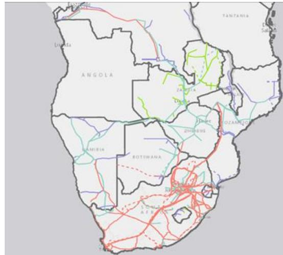
Fig. 1: Map of southern Africa, showing routes of main transmission lines including cross-border interconnectors.
