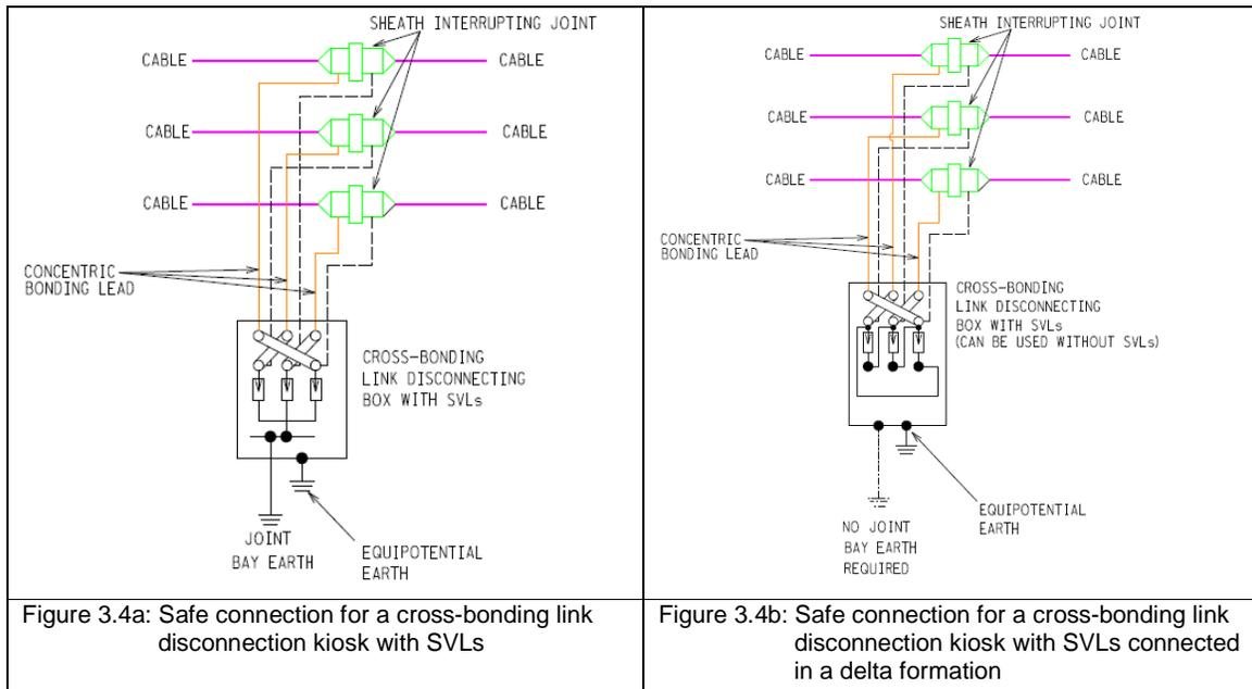
The connections shown in Figure 3.4a are inherently safe, as the HV cable systems earth is separated from the joint bay earth, kiosk housing and equipotential earth through the use of correctly specified SVLs.
