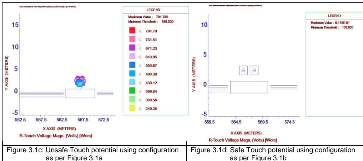
As can be seen from the results FEA results in Figure 3.1c, an unsafe Touch potential is possible and exists if the kiosk's housing is connected to the HV cable system earthing. In order to mitigate against this Touch potential risk, as well as the Step potential risk mentioned in section 2, consider the earthing connection diagram shown in Figure 3.1b.
