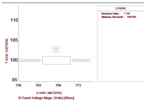
Figure 3.4c: Safe Touch potential using configuration as per Figure 3.4a and 3.4b
