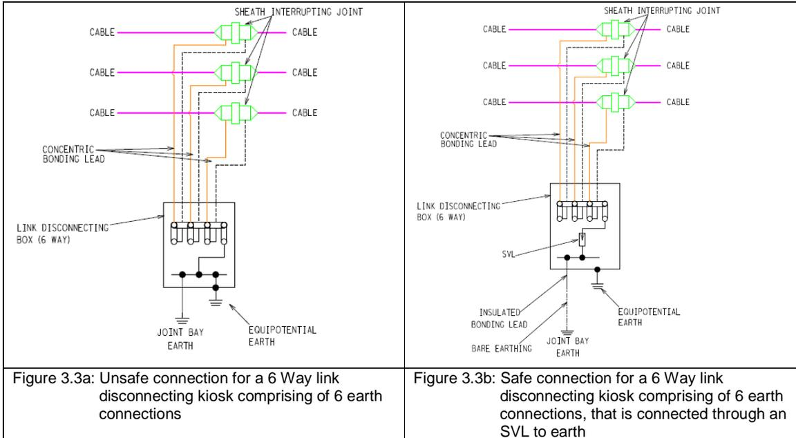
As with the previous case study, an unsafe Touch potential may exist because the housing and joint bay electrode is bonded to the HV cables system earthing.
