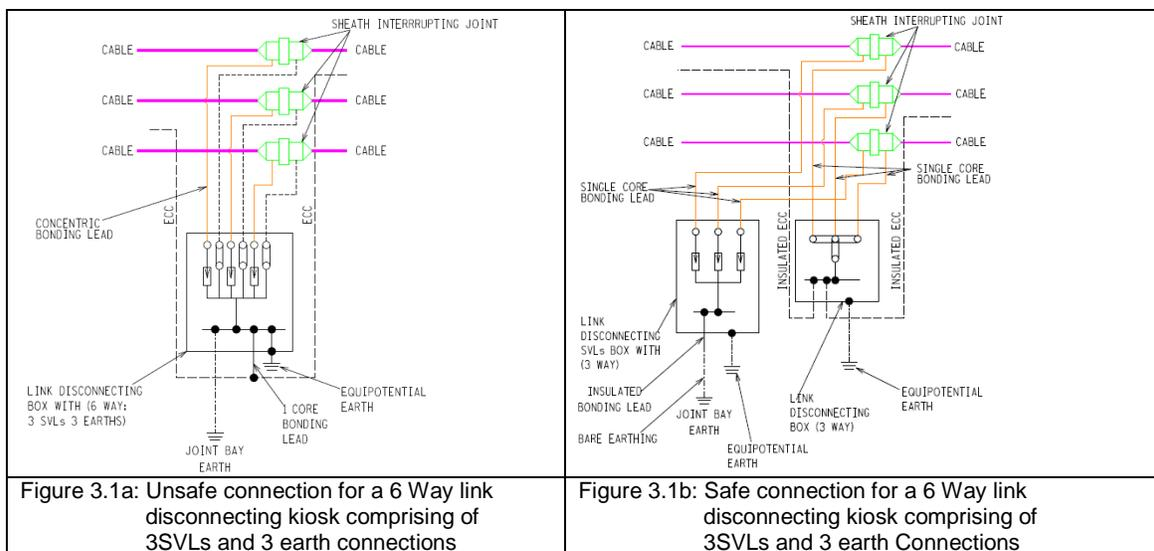
Figure 3.1a: Unsafe connection for a 6 Way link disconnecting kiosk comprising of 3SVLs and 3 earth connections
