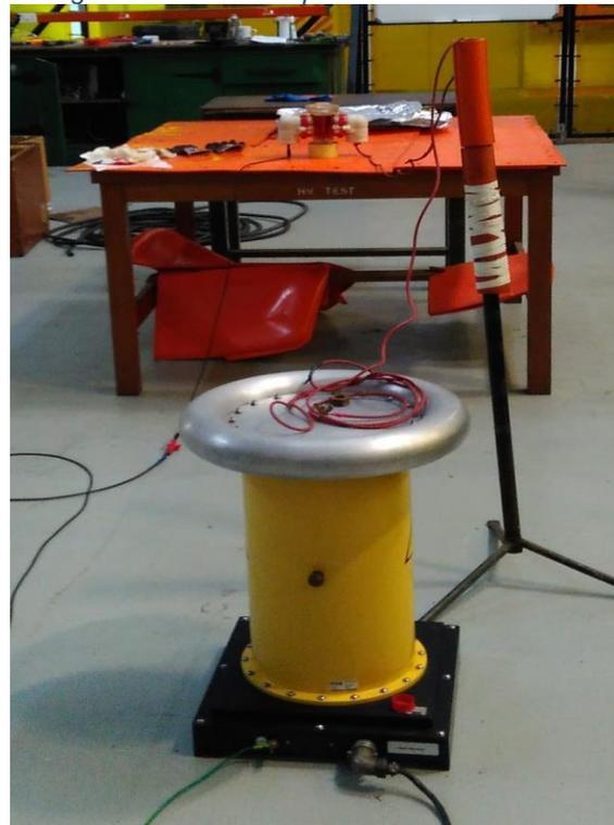
Figure 2: High Voltage Hipot Transformer and lead connections.
