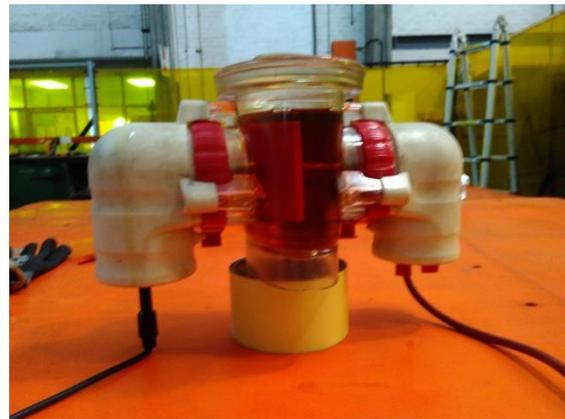
Figure 1: Test vessel filled with insulating transformer oil, 10mm diameter electrodes and a 3D printed specimen. Test leads are from the High Voltage Hipot machine
