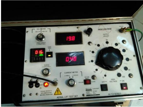
Figure 3: High Voltage Hipot control panel. The manual voltage control can be seen on the right hand side. The top centre display indicates the current voltage level in kV, the lower centre display indicates leakage current in micro amperes. The module on left hand side with display is a timer module.
