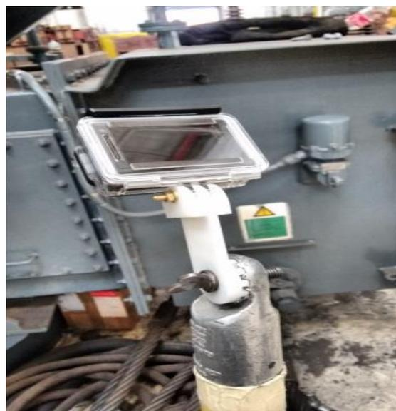
Figure 5: Completed link stick attachment with camera attached
