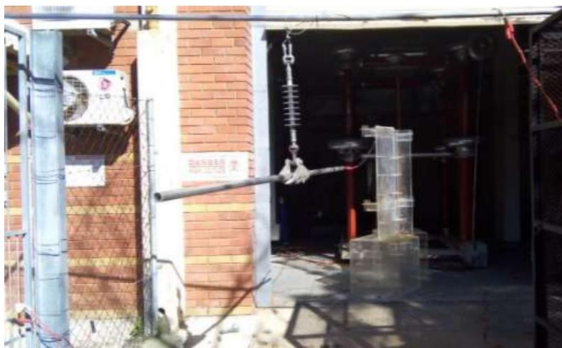
**Figure 2: Photograph of 22 kV SiR insulator setup at the HVDC Lab**
