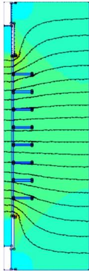
Figure 6: Electric field distribution DC1
