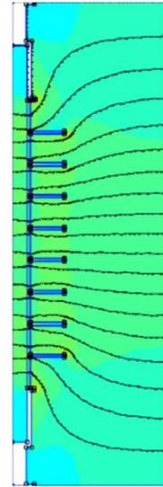
Figure 7: Electric field distribution for DC3
