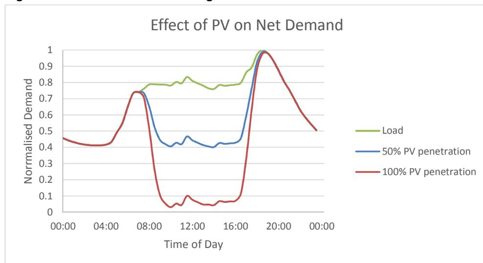
**Figure 4: Effect of PV on Load Duration Curve**
