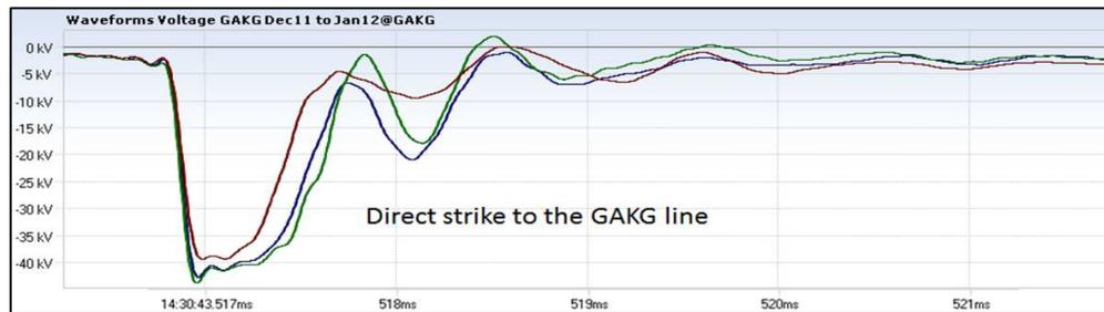
Figure 1-3 Lightning surge on overhead line
