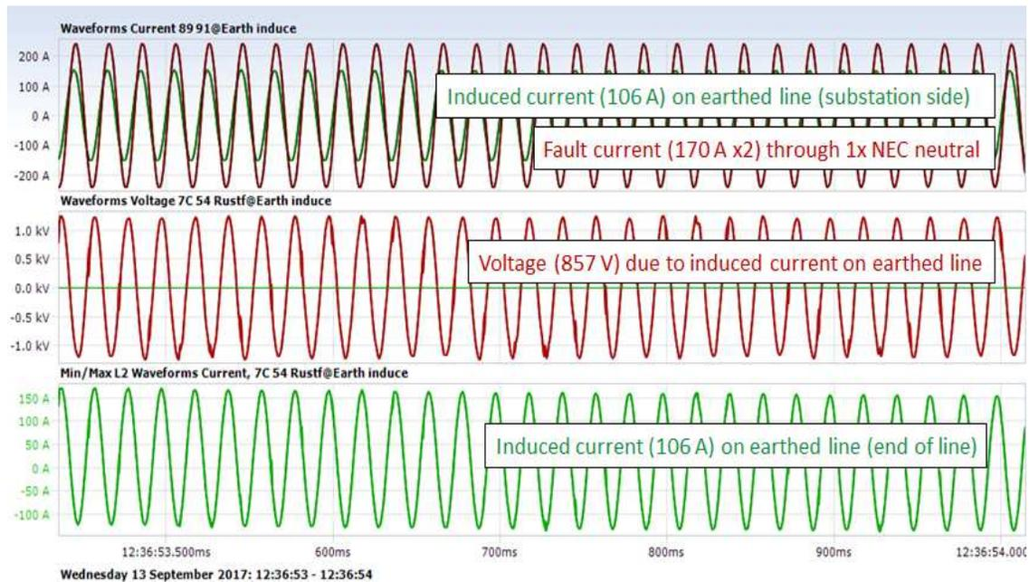
Figure 3-2 Induced voltage and current on parallel line which was earthed at two locations
