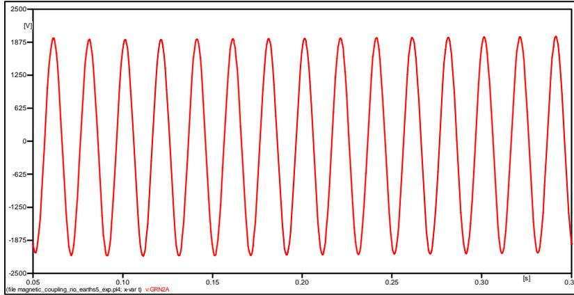
**Figure 2-2 Simulated induced voltage (1390V rms)**
