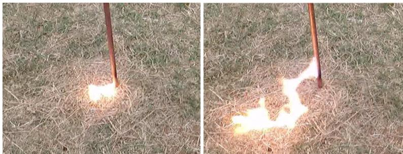
**Figure 1-1 Electrical arc originating from earth spike due to poor electrical connection to earth**
