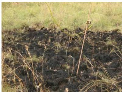
**Figure 1-2 Veld fire caused by fault current flowing to earth via an earth spike**
