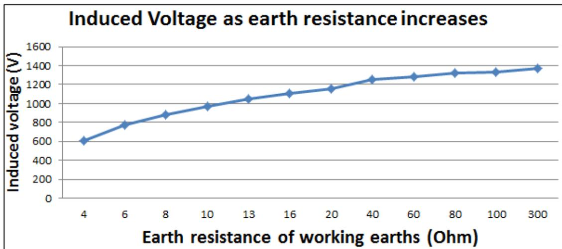
Figure 3-3 Simulated induced voltage at different working earth resistances
