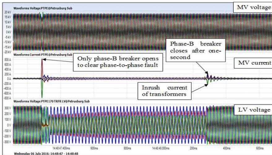
**Figure 3-4 Transient phase-to-phase fault cleared by phase-B single-phase breaker**
