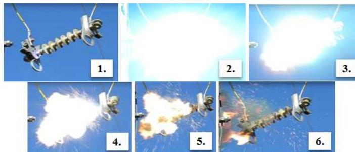
**Figure 3-5 Waveforms of transient phase-to-phase fault as well as photos of the electric arc**
