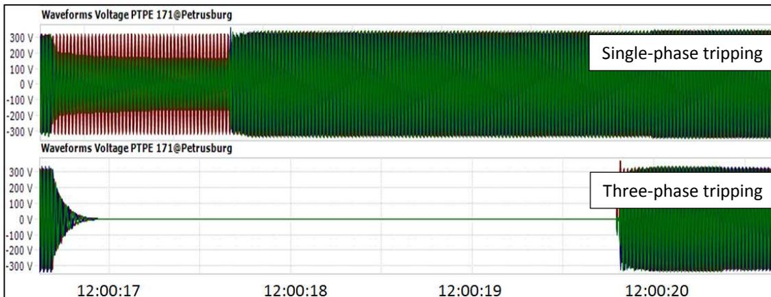
Figure 3-6 Difference between new single-phase tripping philosophy (top) and normal three-phase tripping philosophy (bottom)
