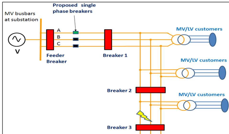
Figure 2-2 Illustration of a MV line with a phase-to-phase fault
