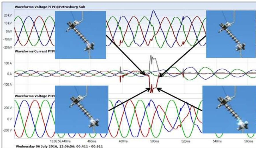
**Figure 3-3 Waveforms of transient earth-fault with electric arc that is barely noticeable**
