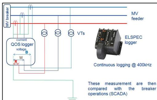
Figure 3-1 Measurement method
