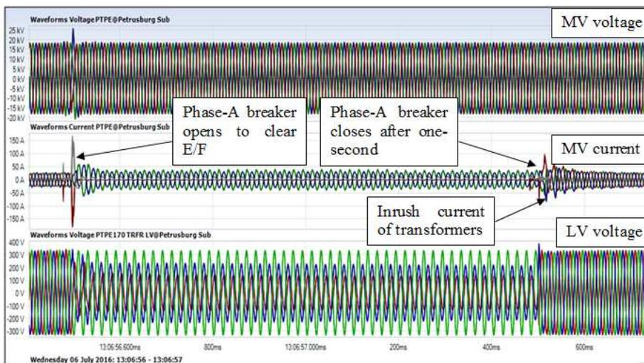
Figure 3-2 Transient earth-fault cleared by single-phase breaker on PTPE line
