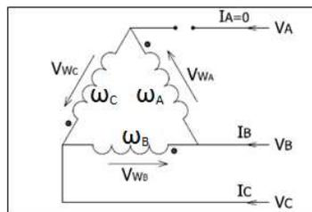
**Figure 2-1 Transformer  $\Delta$  primary winding with phase-A breaker open [11]**
