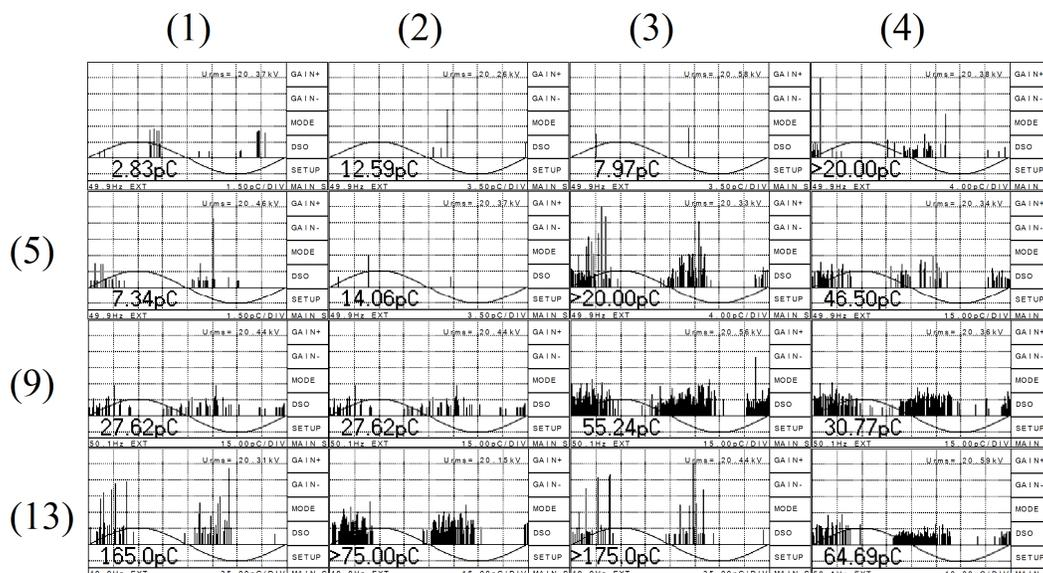
**Figure 1: Clean epoxy PDRP evolution showing single erratic pulses with increasing partial discharge magnitudes for the first four hours. The numbering convention is also shown.**
