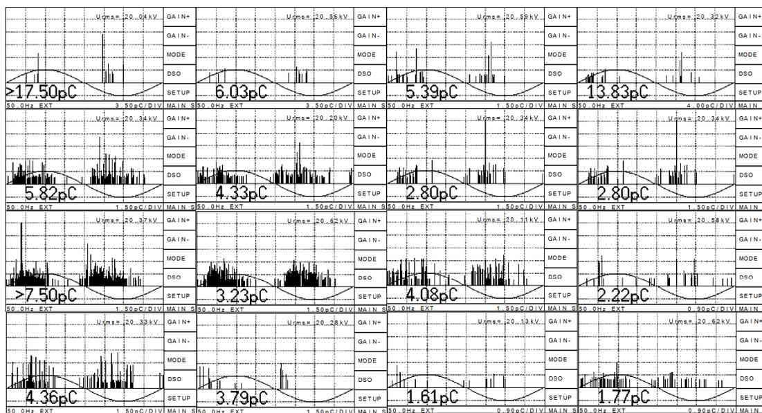
**Figure 2: C/Epoxy 0.33 vol% showing predominantly small and quasi-uniform PD pulses a characteristic of bush tree types.**
