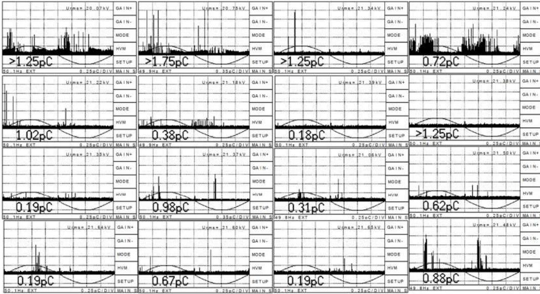
**Figure 3: PDPRPs for BN/Epoxy 1.25 vol% for first four hours showing suppressed PD magnitudes with branch like characteristics.**
