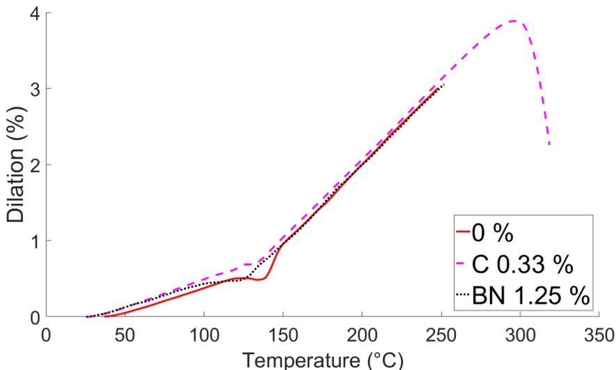
**Figure 4: Thermal expansion results for epoxy, 0.33 vol% C/Epoxy and 1.09 vol% BN/Epoxy.**
