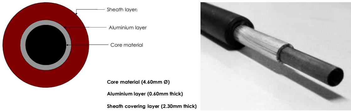
**Figure 1 : Carbon Composite Core Covered Conductor Construction**
