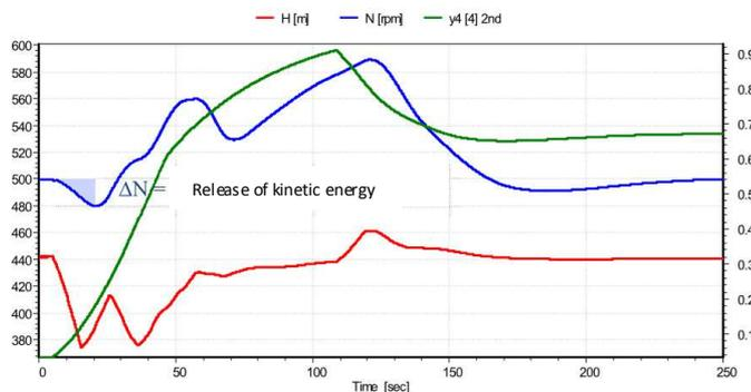
100% power ram up ; (red) water head; (green) turbine opening; (blue) shaft speed
