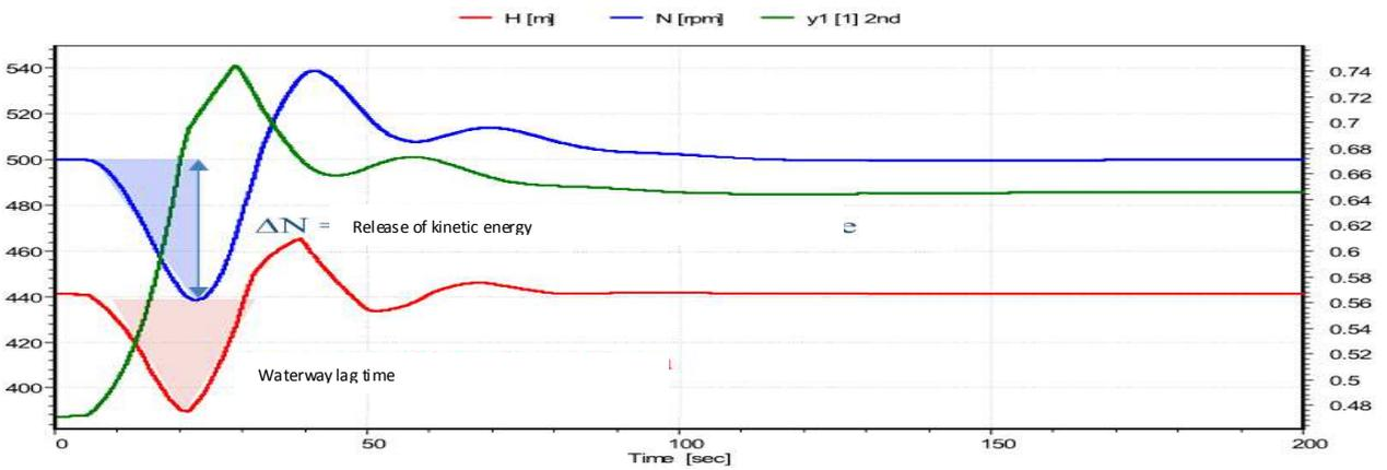
20% power increase: (red) water head; (blue) shaft speed; (green) turbine opening
