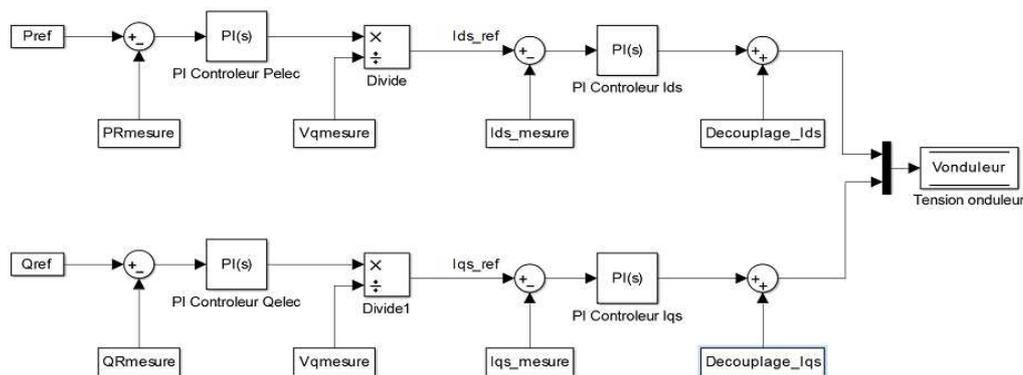
Regulation diagram of the generator side inverter
