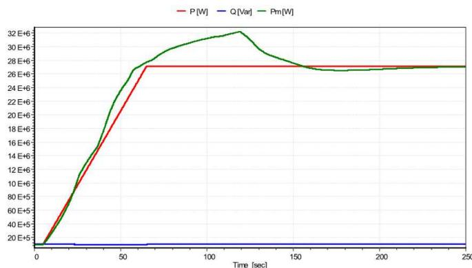
100% power ram up ; (red) Power delivered to the grid; (green) Mechanical power on shaft.
