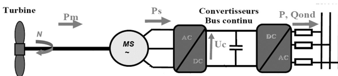
*Schematic diagram of a hydro generator linked to grid through an inverter drive*
