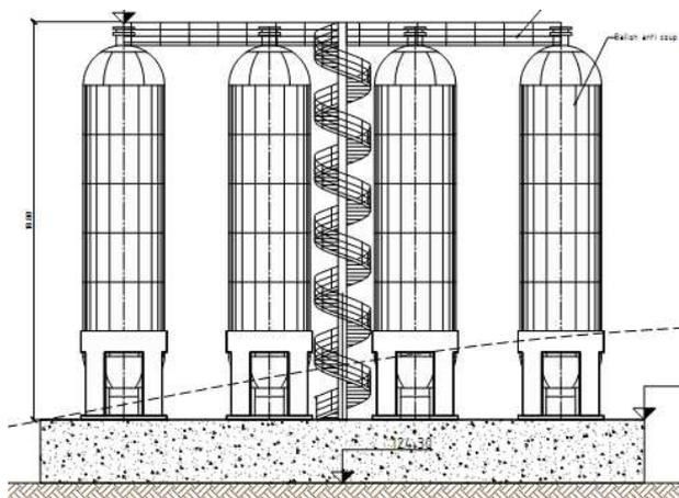
Example of 18m high pressurized tank
