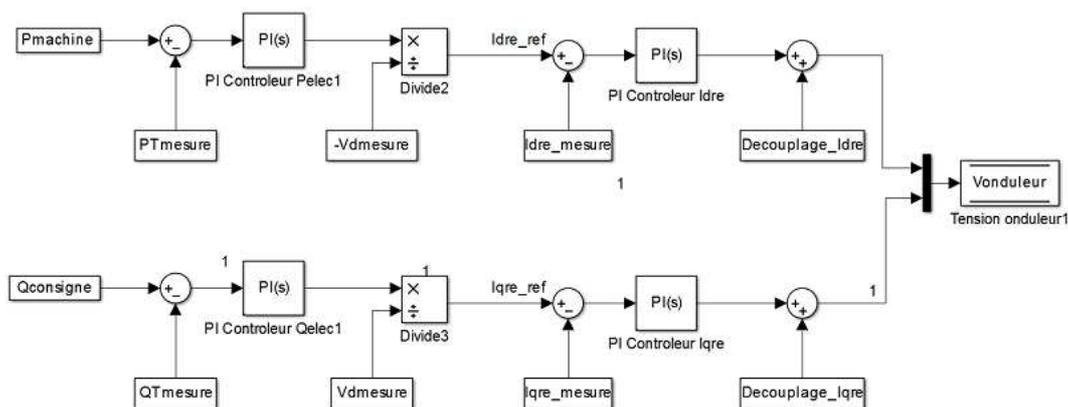
Regulation diagram of the grid side inverter
