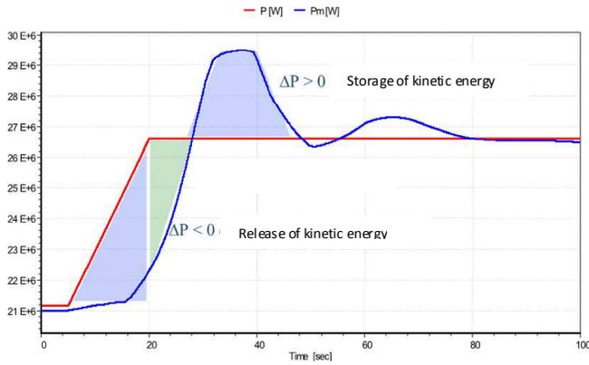
20% power increase: (red) power delivered to grid; (blue) mechanical power on shaft
