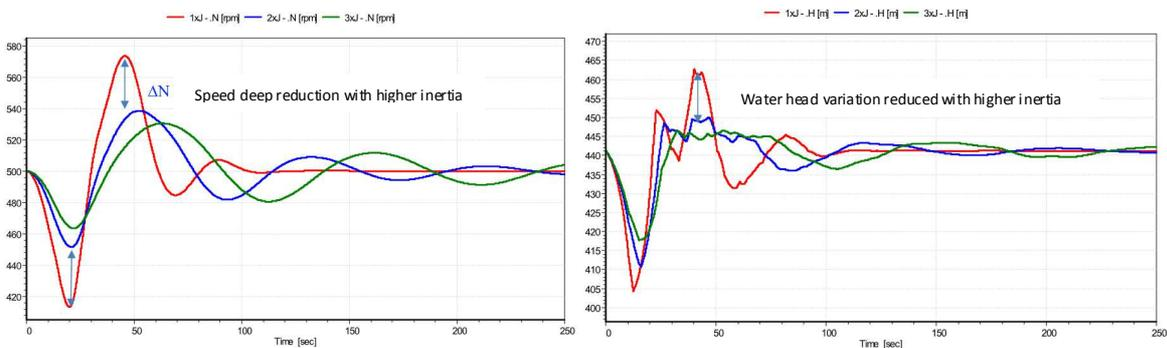
Influence of rotor inertia on speed and water head variation during 20% load ramp up
