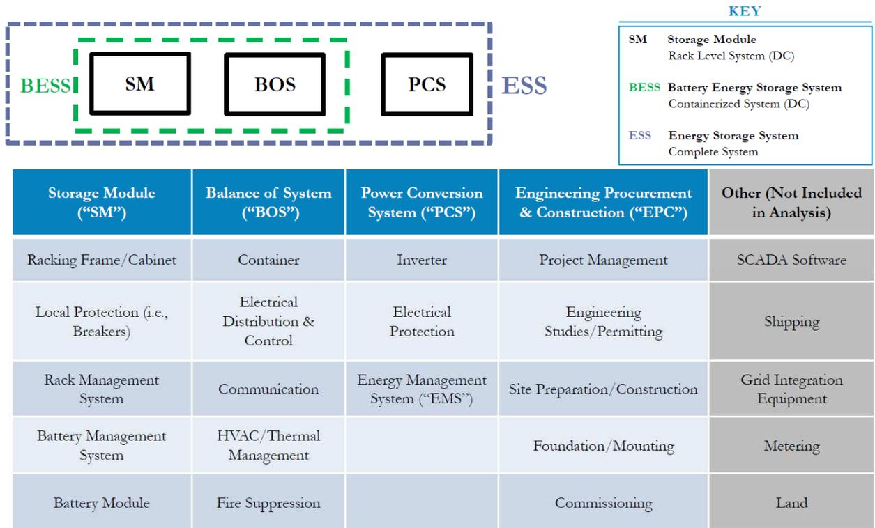
Figure 5 Components making up a full BESS [6]
