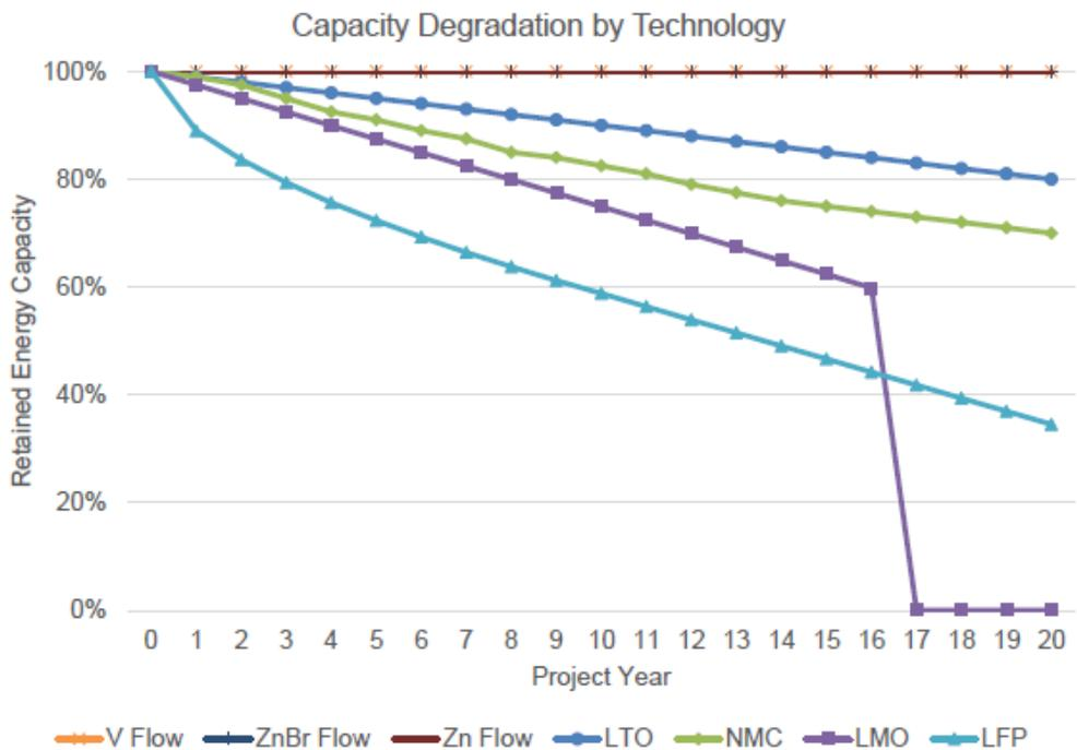
Figure 7 Capacity degradation by storage type and chemistry [5]
