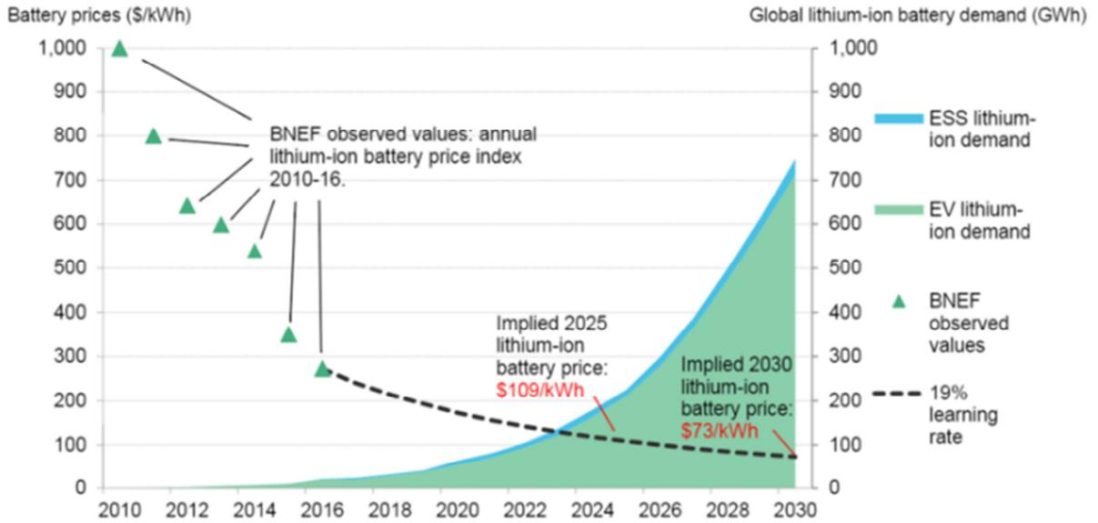
Figure 1 Projected Lithium Ion Battery Prices to 2030 [1]
