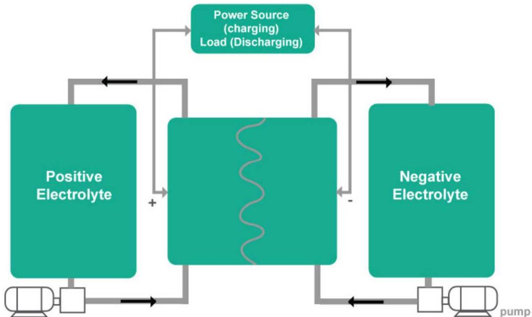
Figure 6 Flow Battery Process [5]
