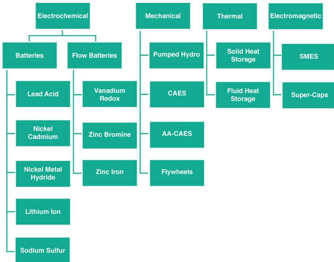
Figure 4 Energy Storage Technologies [5]Error! Reference source not found.
